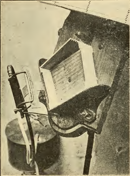
When the foot is in the back position the hot plate is out of the way—nothing to interfere with putting the section in position ready to fold.
